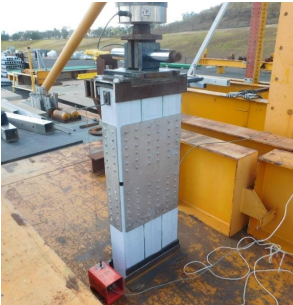
Figure 6. Experimental compressive test setup of the spliced connections
